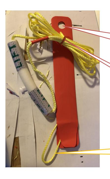
1. Cut hole for attachment to life jacket at the top side with the short lip.
