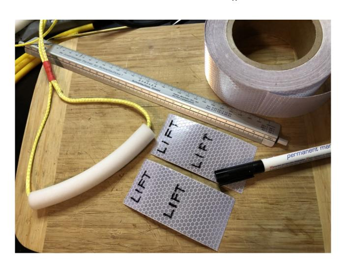
Role reflective tape around the ends of the foam tube in opposite directions so that the instruction "LIFT" can be read from all directions.
