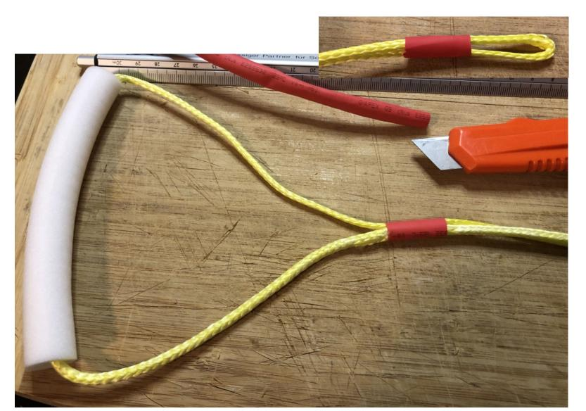
Carefully heat outside of the shrinking tube to lock the triangle for the handle. The dyneema line must not be melted by this outside heating!
