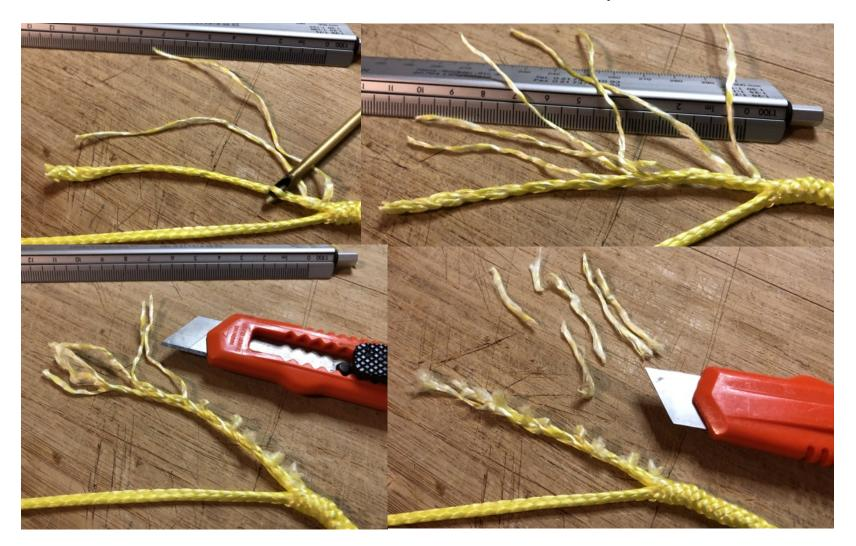
Now again, pull through all slack at the locked joint to the end. Smooth the splice by carefully milking the rope starting at the joint.
